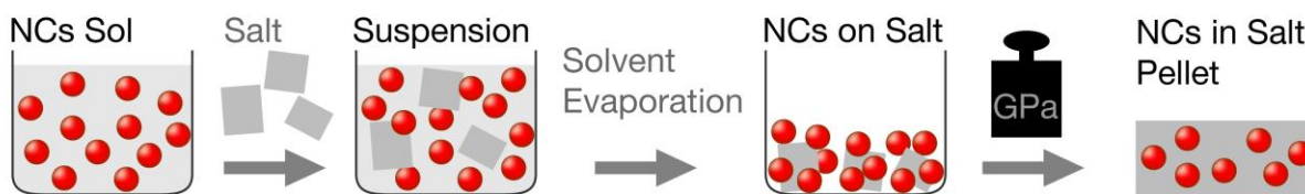
Fig. 1 Scheme for the incorporation of various NCs into NC-salt composite materials using cold flow.
