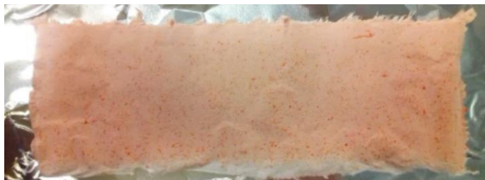
Fig. 1 DOX-PCL nanofibers mat produced by electrospinning
